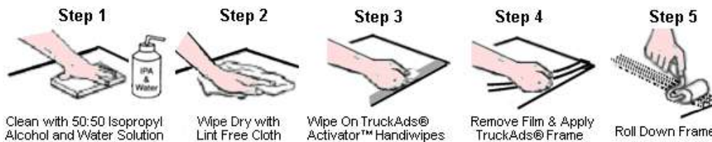
Illustration 3 – Preparing the Surface prior to Installing TRUCK ADS® Clear Frame and Secur-Tabs®
