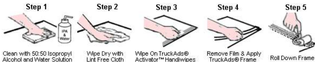
Illustration 13 – Preparing the Surface and Installing TRUCK ADS® Black Frame
