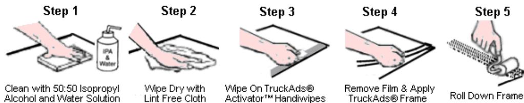
Illustration 13 – Preparing the Surface and Installing TruckAds Black Frame™
